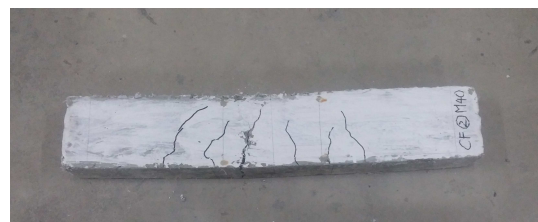
Fig. 10. Flexural failure of fiber-reinforced beam
