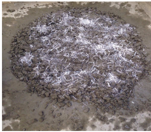
Fig. 2. Addition of fibres in concrete mix.
