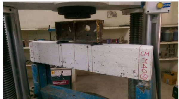
Fig. 9. Test setup for RC beam.
