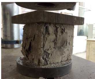
Fig. 3. Testing of cube specimen.
